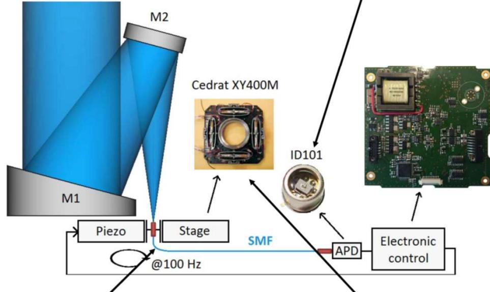
SOLUTION 1: Baffling : use of single mode fiber
