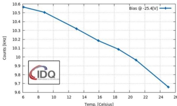
Detection as function of temperature of detector
